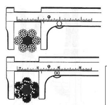
The upper illustration shows the correct method to measure wire rope. Note that the strands are oriented such that the rope's maximum width is measured.
